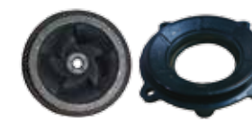
High chrome enclosed impeller Heat treated ductile-iron suction plate AISI 410 Heat treated shaft (Optional for customized request)
